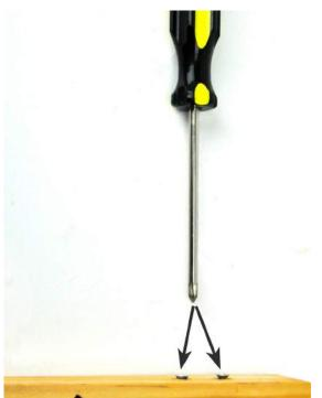
Step 4: Securely hold the Wooden Rack Foot (B) to the Wooden Rack (A) and using Small Philips Screw Driver, screw the Screws (C) until the screws pierce into the bottom of the Wooden Rack (A) and securely hold in place. Repeat this step for the other Wooden Rack Foot (B).
