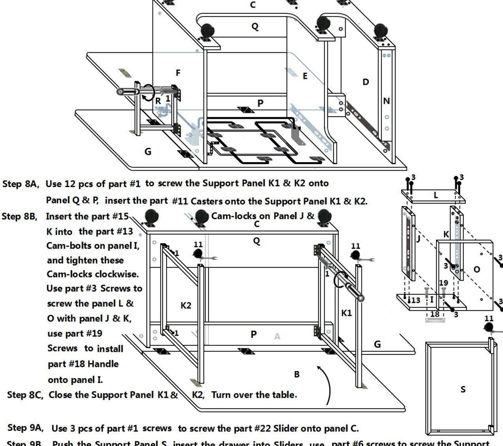
Step 9B, Push the Support Panel S, insert the drawer into Sliders, use part #6 screws to screw the Support
